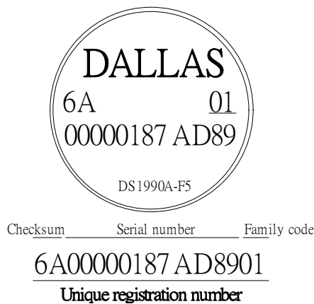
Fig1. Touch Memory Button from Dallas Semiconductor and it'sunique 16-character registration number.
