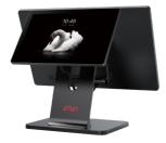
More capabilities Built-in NFC module on secondary display to provide a seamless payment process.
